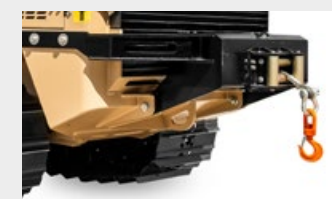
Rear winch with 6 t pulling power
